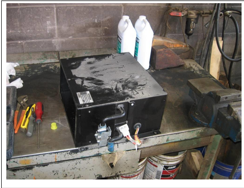
With heater box on a work bench remove the lid.
